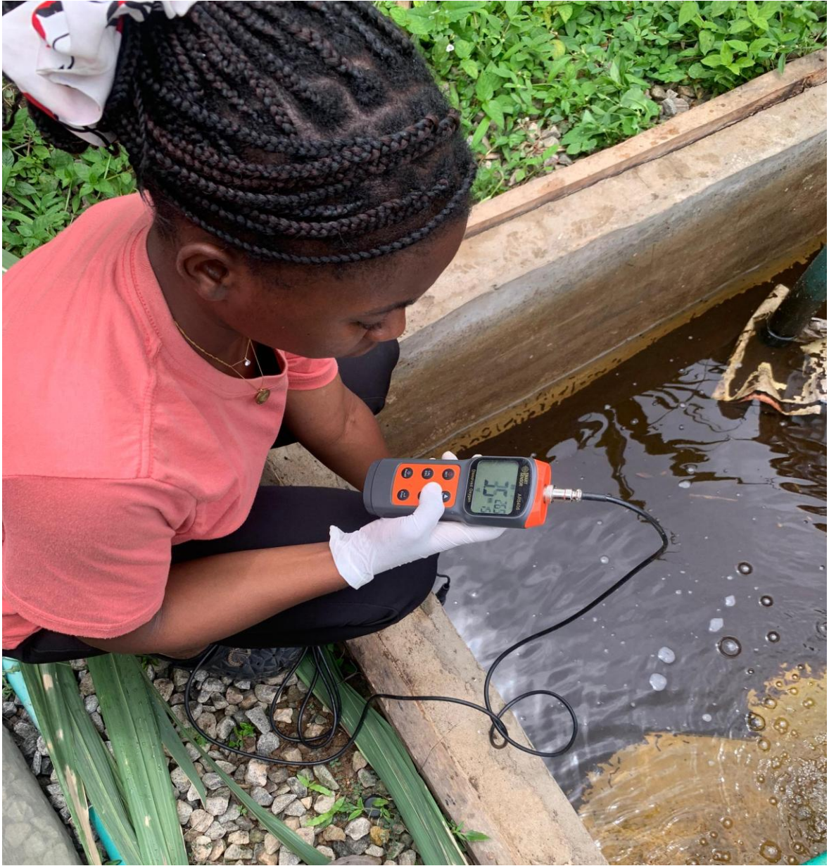
Plate 1: Measuring the dissolved oxygen concentration in sump water at INCiTiS-FOOD Living Laboratory.
