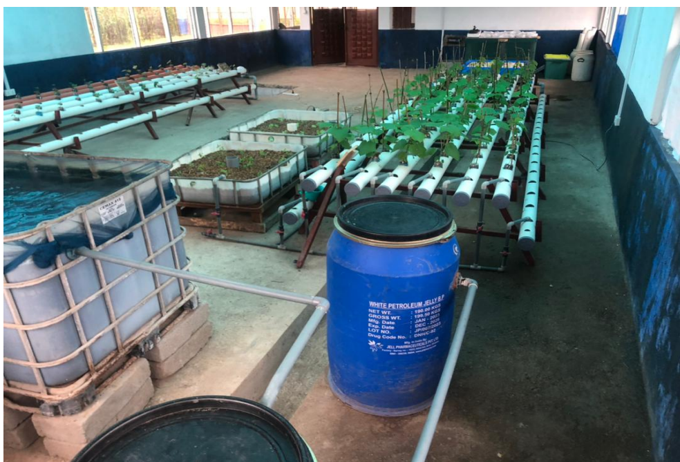
Figure 3.2. Image of the experimental setup showing the IBC tank where fish was raised
